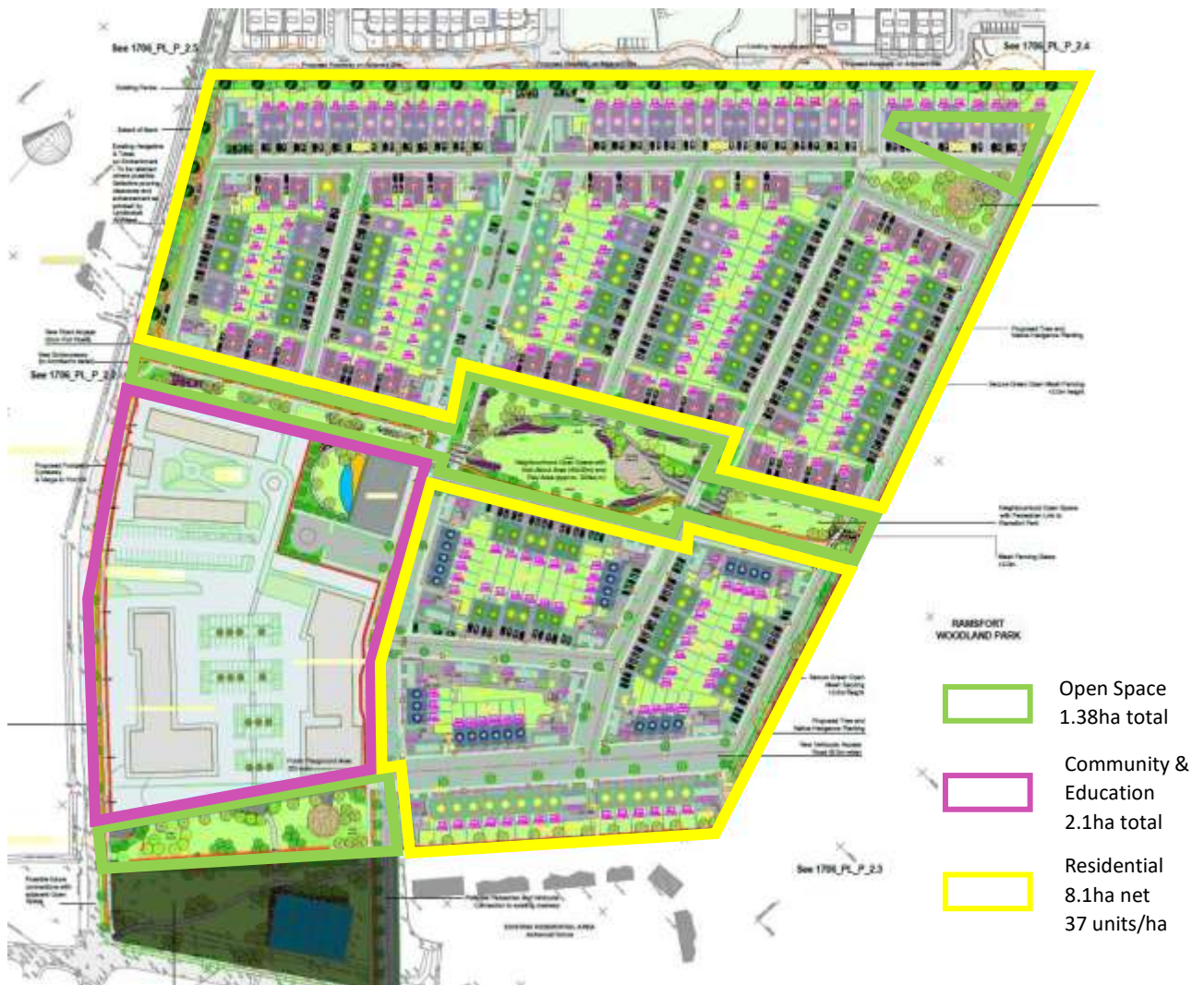
Site Layout highlighting Open Space provision, Areas & Residential Density, with indicative masterplan for Community & Education zoned lands
